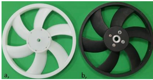
Figure 1. Photographies of (a) a rotational moulded fan and (b) the reference aluminium machined fan
