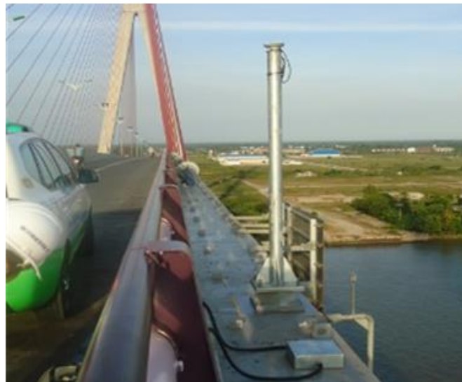
Figure 7. GPS rover on girder location.
