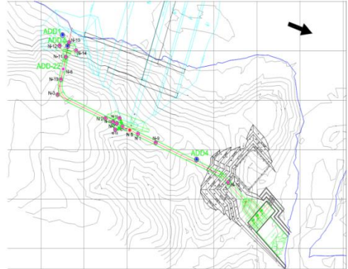
Fig 5. Drill hole location along Waterway Tunnel
