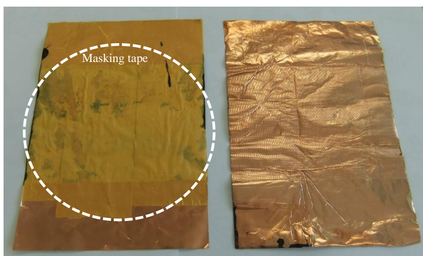
Fig. 8 Coated surface before and after the masking tape is removed.
