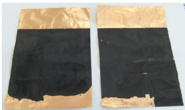
Fig. 6 Anode and cathode sheets after coating.
