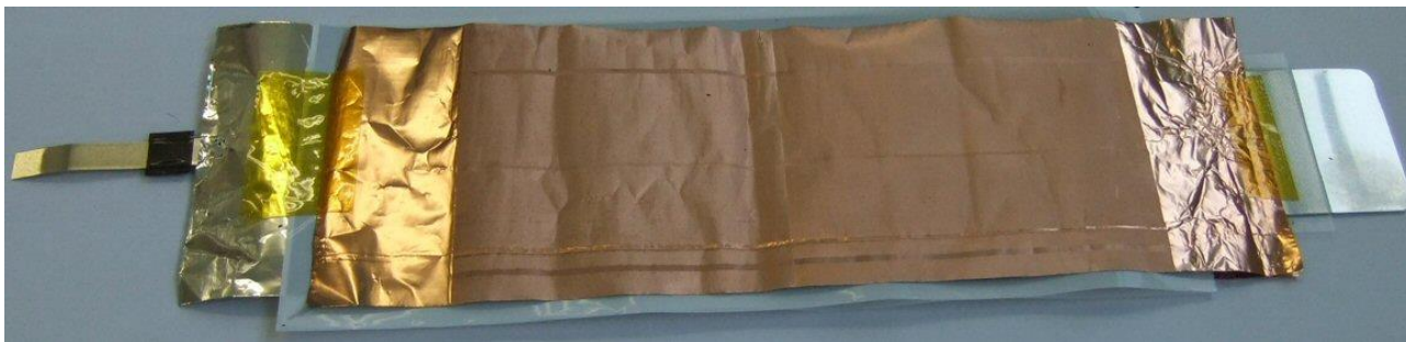
Fig. 14 Electrode body before sticking lithium metal foil.
