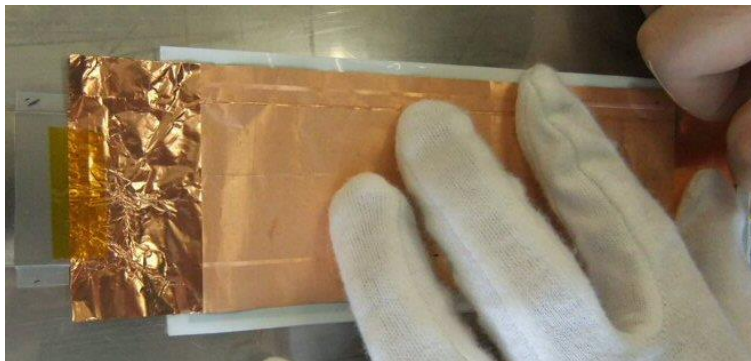
Fig. 13 Assembling electrode body with separator.
