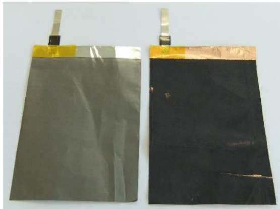
Fig. 10 Negative and positive electrode sheets each with a tabbed lead.
