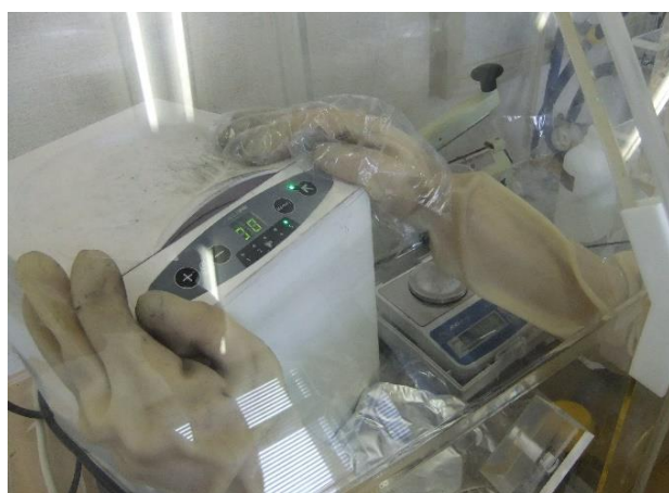
Fig. 17 Mixing and stirring work by planetary system.
