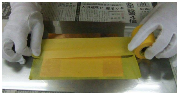
Fig. 7 Pasting work the masking tape onto the current collector before coating.
