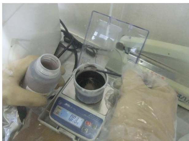
Fig. 16 Weight measurement of lithium metal powder.
