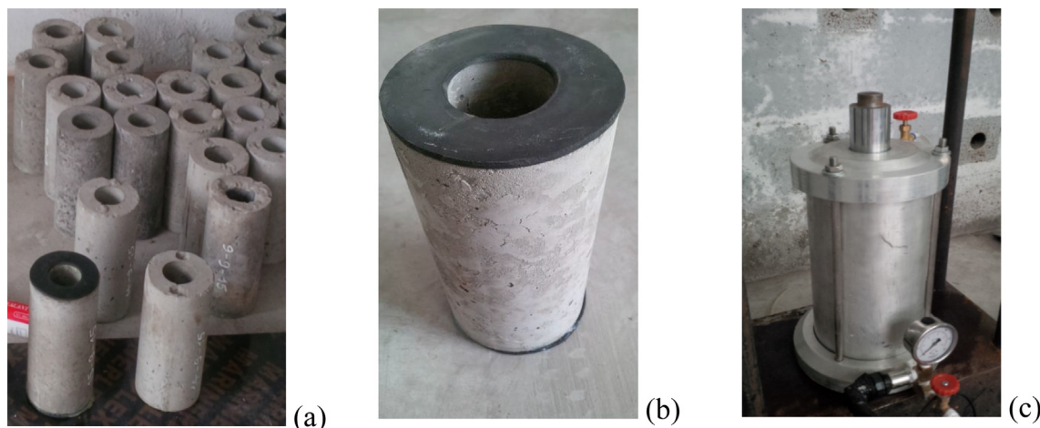
Fig. 2. Hollow cylindrical concrete samples for water permeability test (a, b); permeability cell (c).
