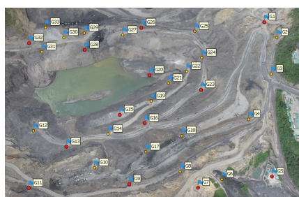
Fig. 3. Distribution of GCP of the studied area in the Dong Da Mai mine, Quang Ninh
