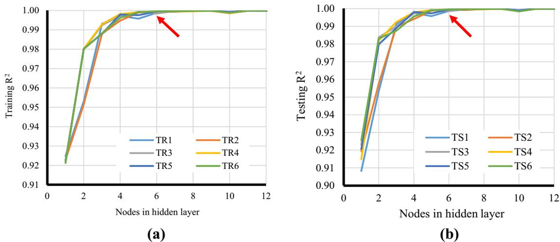
Fig. 7  $R^2$  variation against the nodes number in terms of the prediction of bearing capacity
