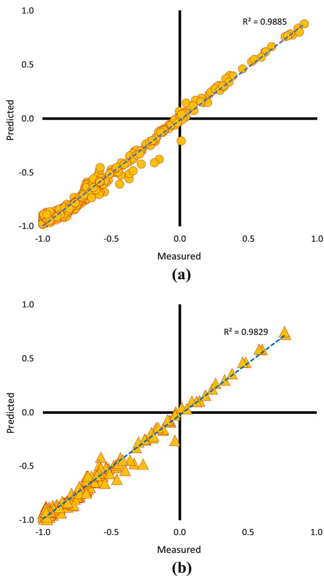
**Fig. 12** Training and testing outcomes obtained by ALO–MLP model in terms of predicting shallow circular footing bearing capacity
