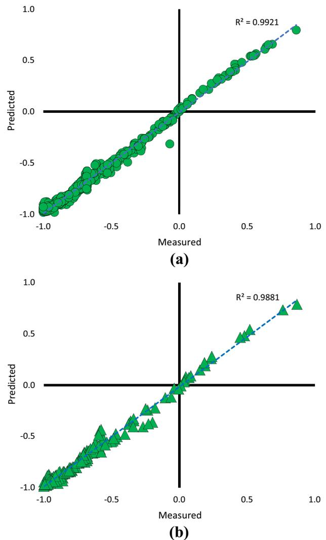
**Fig. 11** Training and testing outcomes obtained by SHO–MLP model in terms of predicting shallow circular footing bearing capacity
