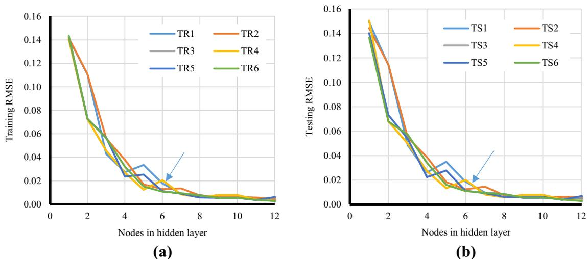
Fig. 8 RMSE variation against the nodes number in terms of the prediction of bearing capacity
