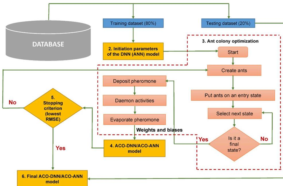
Fig. 4. Global search of the ant colony and optimization of DNN (ANN) by the ACO algorithm.
