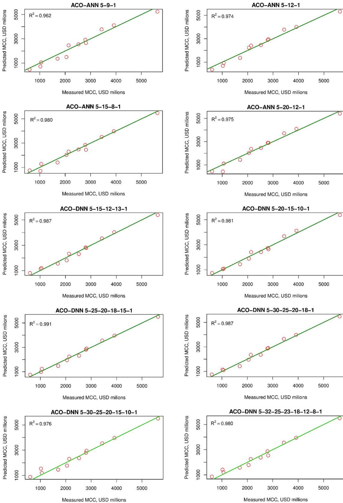
Fig. 18. Testing performance of the ACO-ANN and ACO-DNN models.
