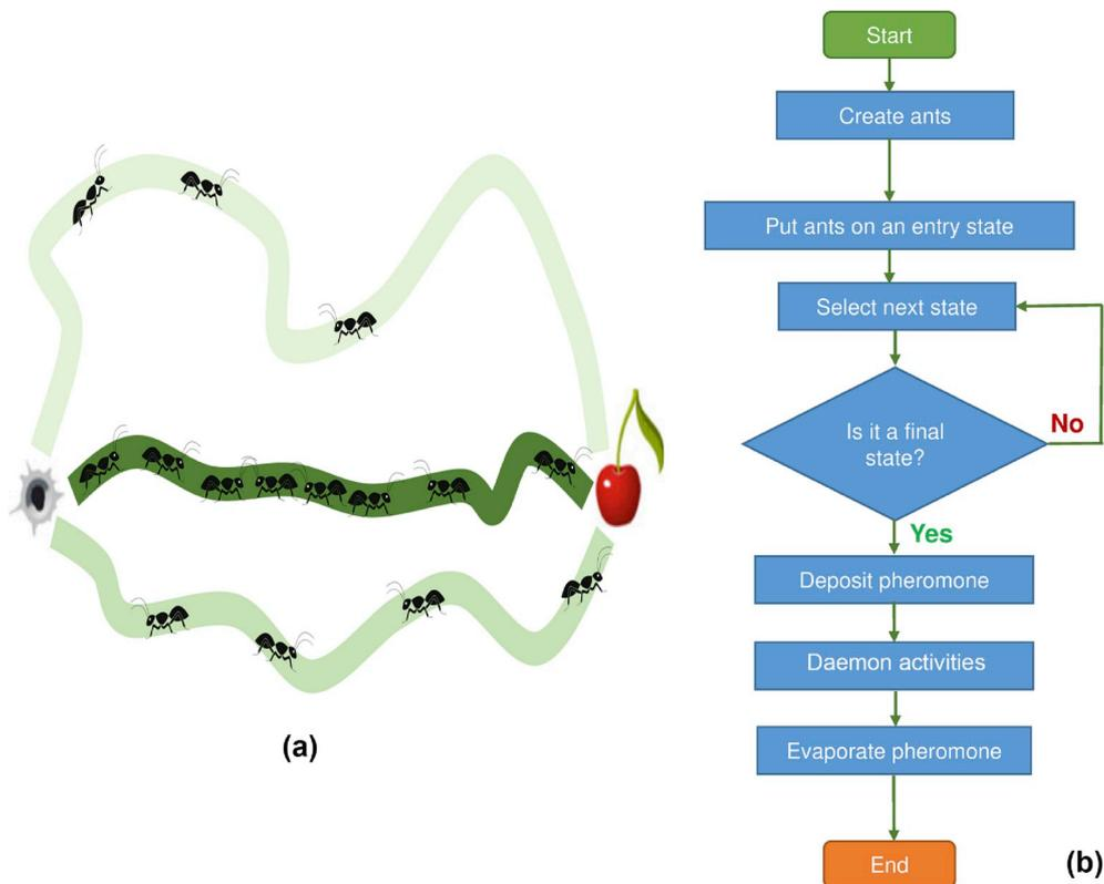
Fig. 2. Paths and pheromone of ants and their flowchart. (a) Paths of ants and the amount of corresponding pheromone (Mirjalili, 2019); (b) Flowchart of the ants for optimization.
