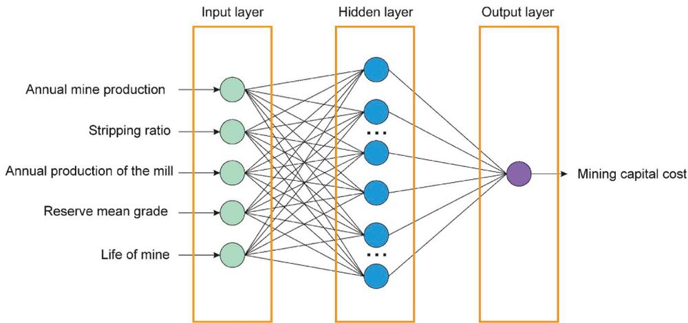
Fig. 3. General architecture of ANN/DNN for predicting the CC of mining projects in this study.
