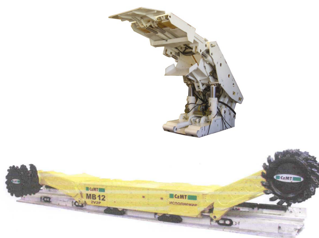
Fig. 3. Support VINAALTA 2.0/3.15 and shearer MB 12-2V2P/R-450E applied at Vang Danh coal mine in period of 2008–2012.
