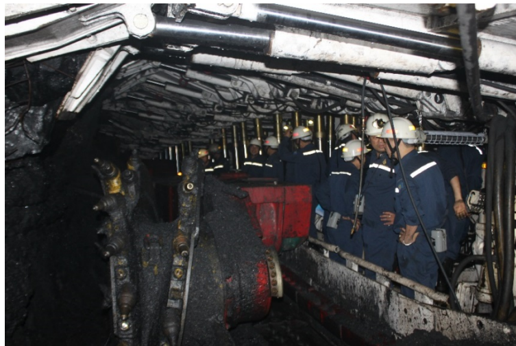
Fig. 5. Support ZF4400/16/28 and shearer MG 150/375-W applied at Ha Lam coal mine.
