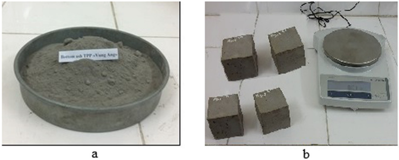
Fig. 2. a - Bottom ash TPP «Vung Ang», b - Determine the weight of concrete specimens.
