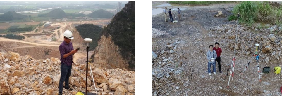
Fig. 3 GCP marks and their coordinates measured by GNSS/RTK
