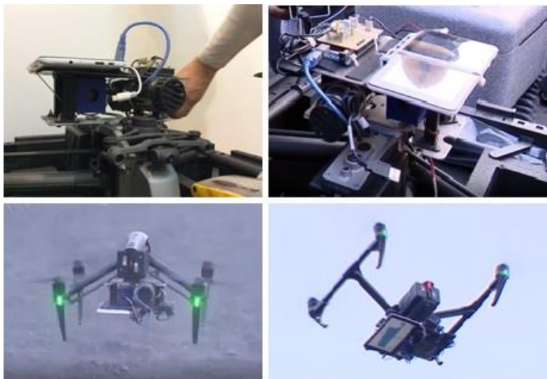
Fig. 3. Air quality monitoring components of the UMS-AS system
