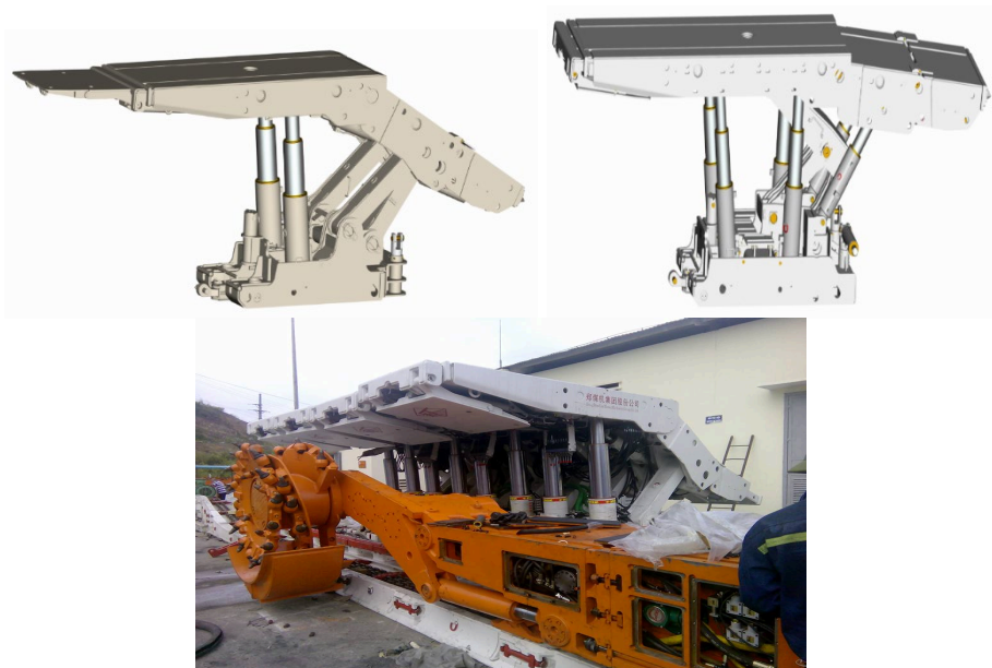
Fig. 6. Supports ZFY5000/16/28, ZFG6200/17/30 and shearer MG150/375-WD applied at Khe Cham III coal mine since 2016.
