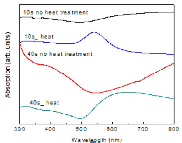
Figure 3. Absorption spectra of gold thin films with and without heat treatment.
