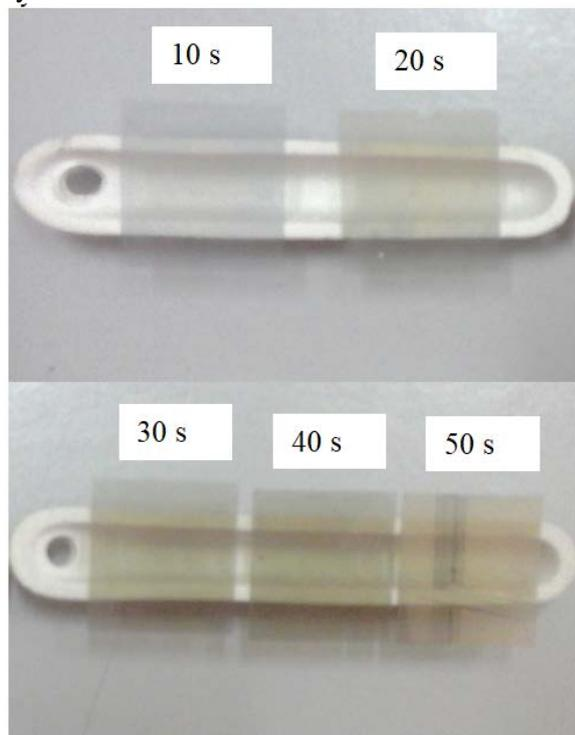
Figure 1. Image of gold nanoparticles array prepared by sputtering and thermal annealing method. The sputtering time is 10s, 20s, 30s, 40s and 50s.
