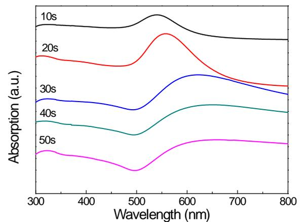
Figure 5. Absorption spectra of gold thin films prepared by sputtering method after heat treatment.
