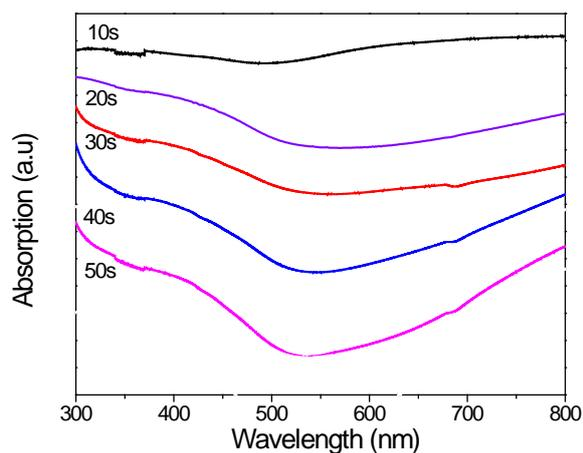
Figure 4. Absorption spectra of gold thin films prepared by sputtering method.
