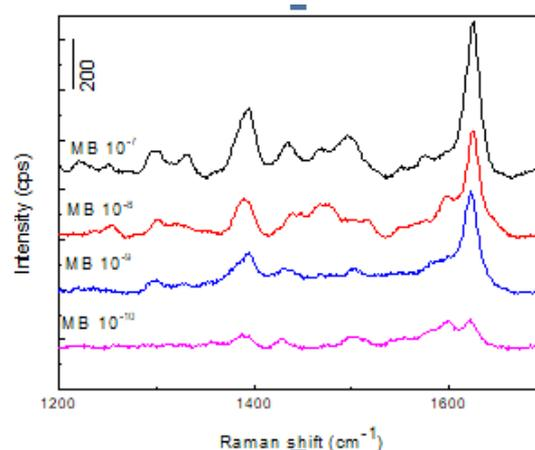
Figure 4. Raman spectra of methylene blue adsorbed on gold nanoparticles prepared from gold thin films sputtered in 40s.
