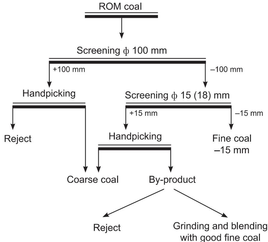
**Figure 4:** Simple treatment system for ROM coal at coal mines
