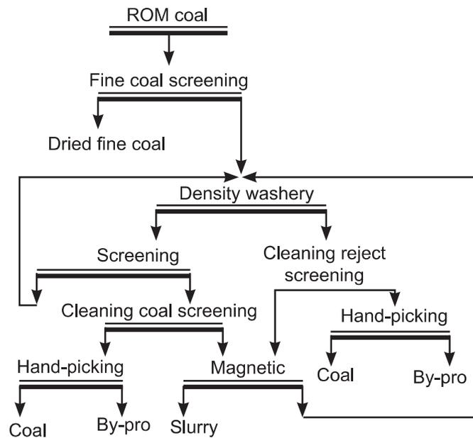
Figure 6: Flowsheet of Vang Danh coal processing plant (Viet Bach and Gheewala, 2008)
