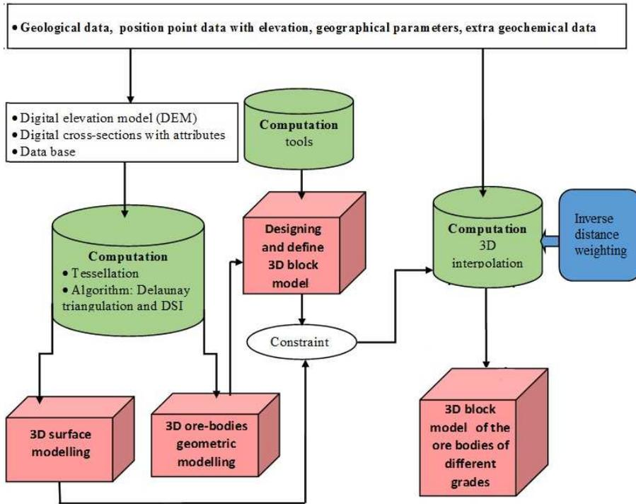
Fig. 3. The block scheme of 3D modeling process.
