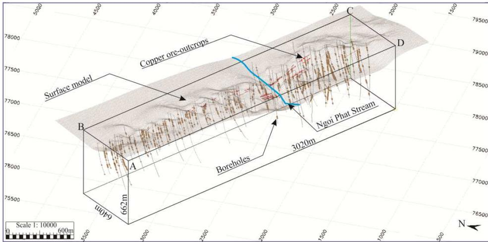
**Fig. 6.** The surface model of the studied area.
