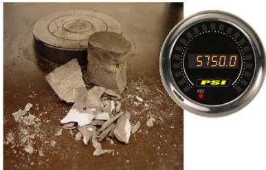
Figure 7. Conventional cement sheath with catastrophic failure
