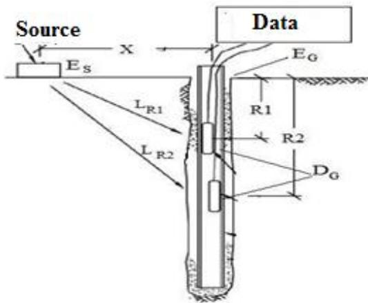
Fig. 2. Diagram calculating in the downhole seismic testing method
