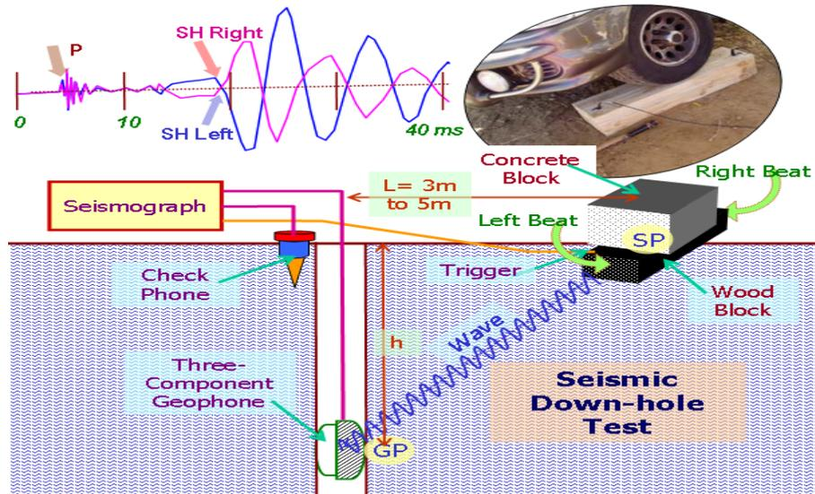
Fig. 1. Diagram of downhole seismic testing
