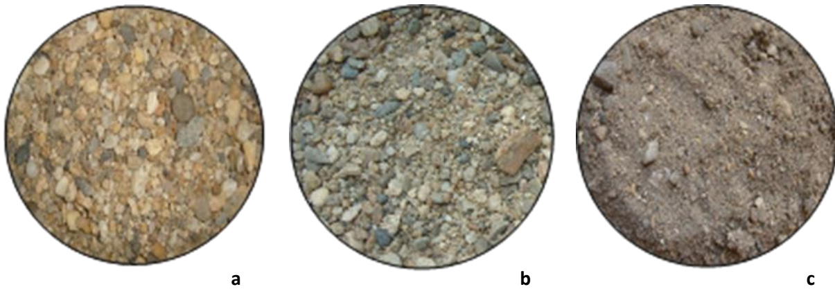
Fig. 5. Types of material used for the physical model a. Pebble b. Pebble mixes with sand c. Sand (moderate grain size) mixes with pebbles
