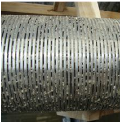
Fig. 10. The wire-winding pipe (a) and slit pipe (b) after experiments.
