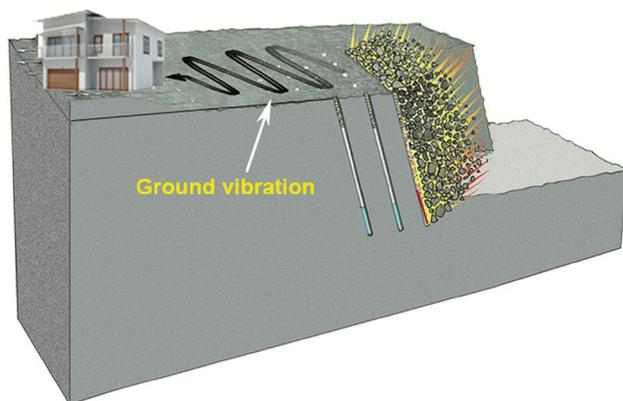
Fig. 1 Blast-induced ground vibration for rock fragmentation
