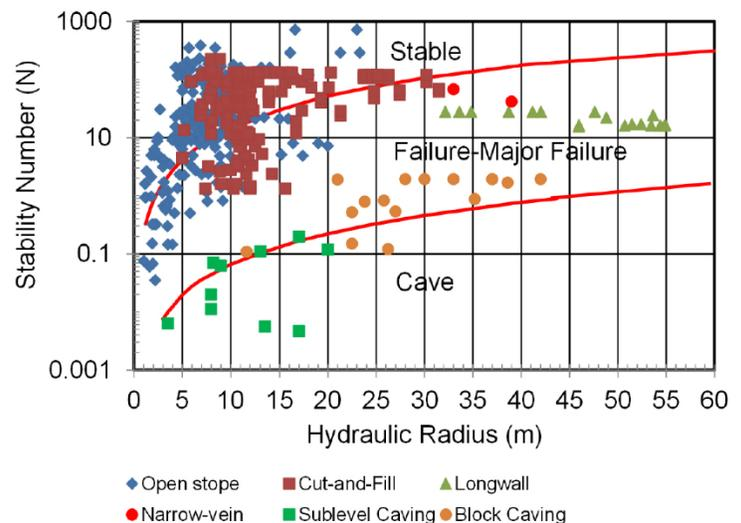
Fig. 8 Composition of the extended Mathews stability graph database by mining method (Suorineni, 2014).
