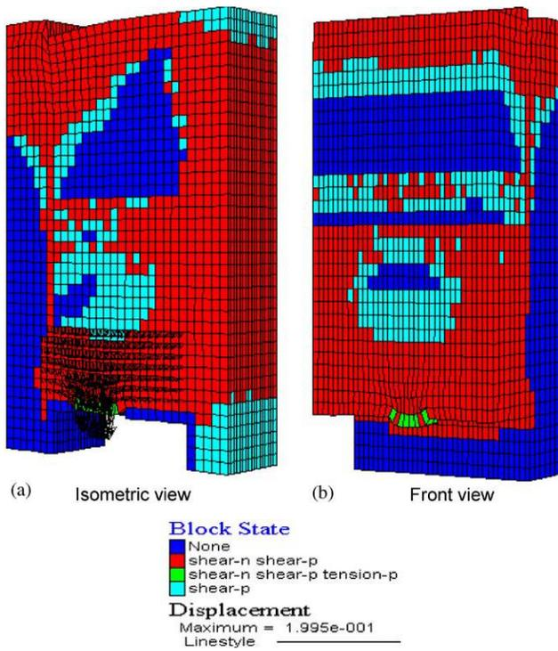
Fig. 4 Vertical state of coal failure during caving (Yasitli and Unver, 2005).
