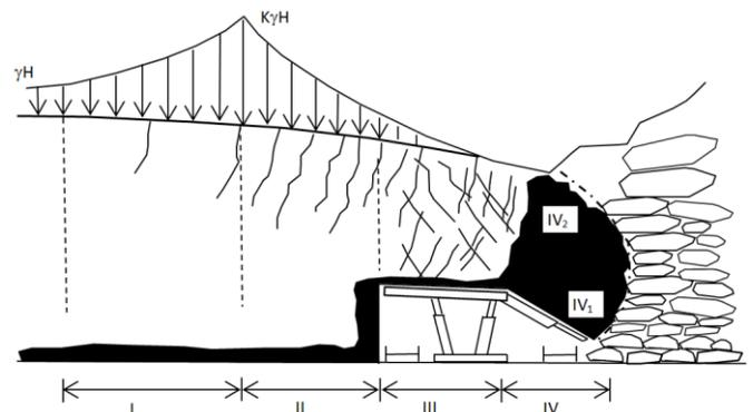
Fig. 6 Coal seam deformation and fracturing in LTCC mining (Humphries et al., 2006).
