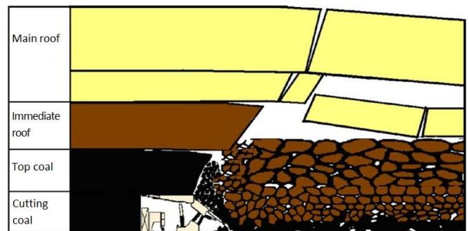
Fig. 1 Roof strata in Longwall Top Coal Caving face (Vakili, 2009).
