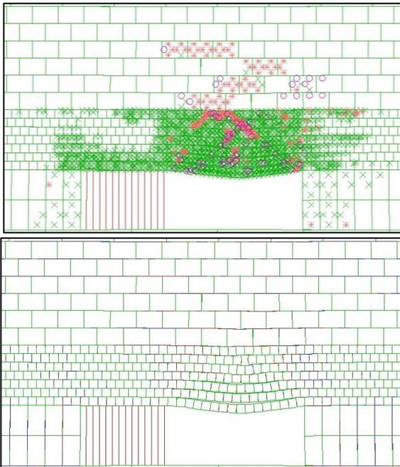
Fig. 7 Failure in top coal before first caving (Le et al., 2017b). NOTE: blocks that fail in current shear, past shear and tension are illustrated by red star \*, green X and purple o, respectively; discontinuities that have opened and slipped are in red and blue colour, respectively.
