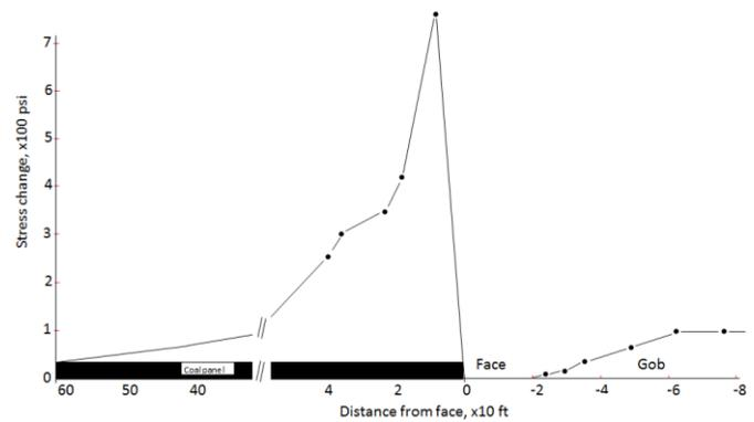
Fig. 3 Front abutment stress versus SPL face distance (Peng and Chiang, 1984).
