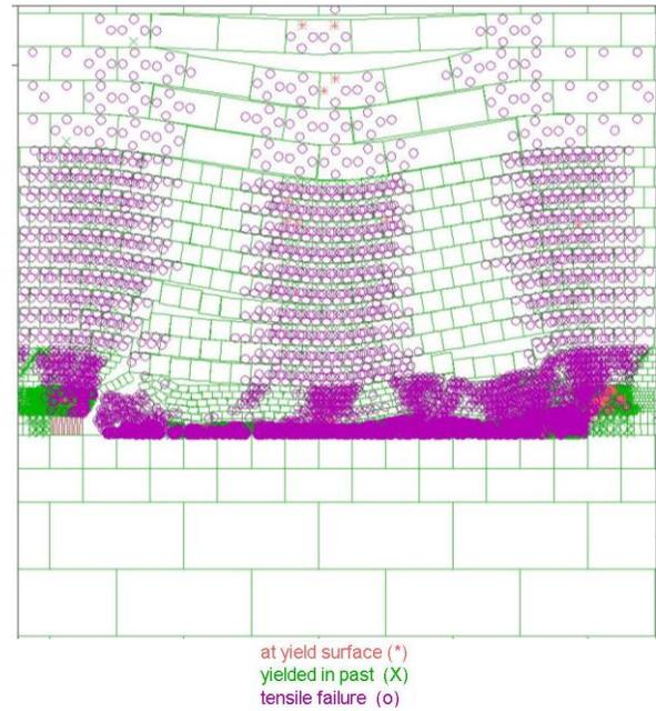
Fig. 5 Rock block failure in the first weighting of roof strata (Le et al., 2017b).
