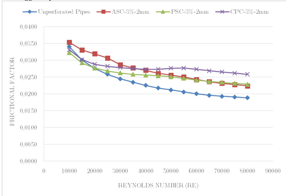
Figure 2: Friction factors in pipes with 3% perforation ratio, 2mm size
