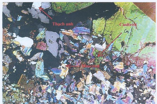
Figure 3. Greisenized granite, The thin section petrology sample KTD.288, nicol (+), x 35.
