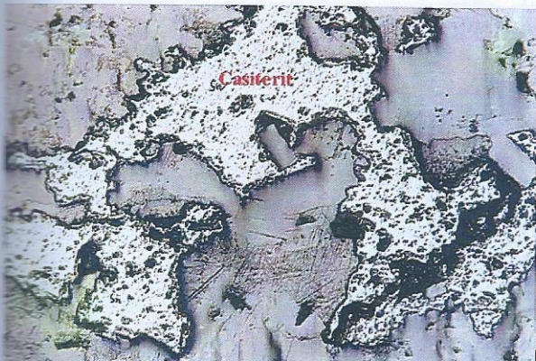
Figure 6. The mineragraphic sample KTD. 1575x50, cassiterite.
