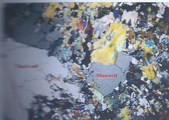
Figure 2. Greisenized granite - The thin section petrology sample M.143, nicol (+) x 35.
