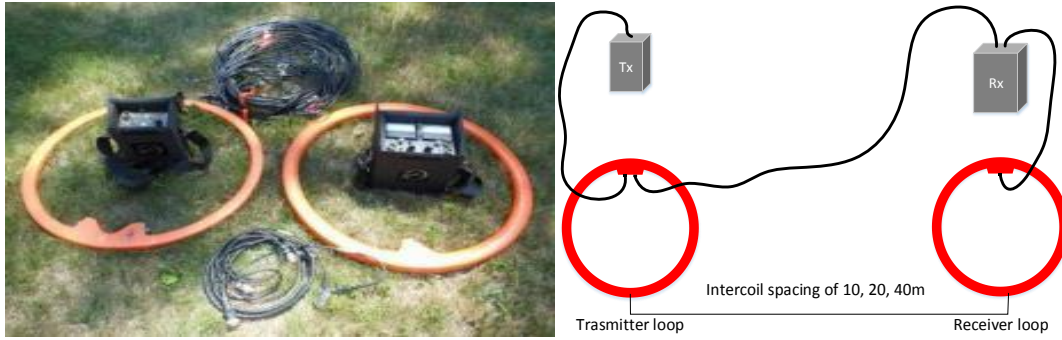
Figure 1. Geonics Electromagnetic EM34-3 instrument applied in study area
