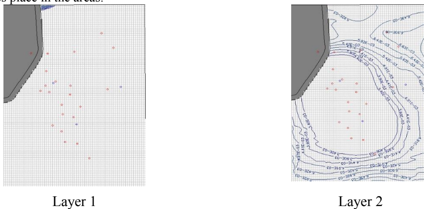
Figure 4. Simulation of compaction in the Layer 1 and Layer 2 in MaiDich water plant
