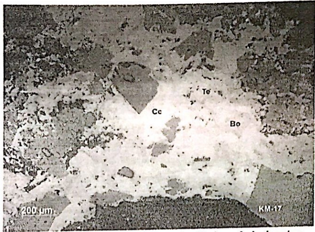
Figure 6. Tetraedite (Te), bornite(Bo) and chalcocine (Cc) nest disseminated ores in host rocks of Khuon Muoi copper mine.
