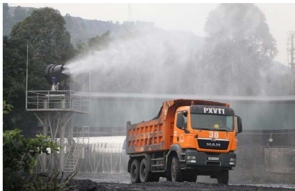
Figure 8: The high-pressure moisture sprayer in Coc 6 Coal Mine helps reduce dust on the company surface
