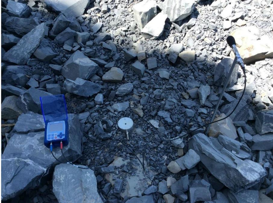
Figure 10. Micromate device and AOP measurement by the microphone.
