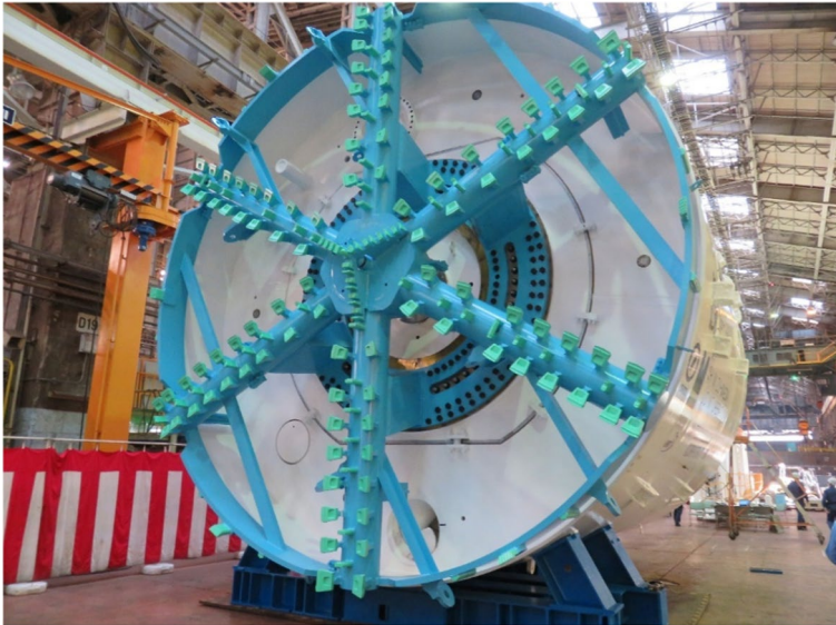
Fig. 2 Excavation face of the EPB TBM in Ho Chi Minh Metro Line 1
