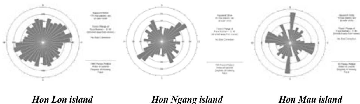
Figure 6. Rose diagram of fracture systems on Hon Lon, Hon Ngang and Hon Mau islands.
