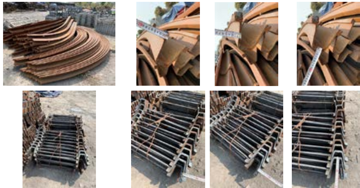
Figure 12. U-beams employed in tunnels and the measurement of their dimension using a tape.
