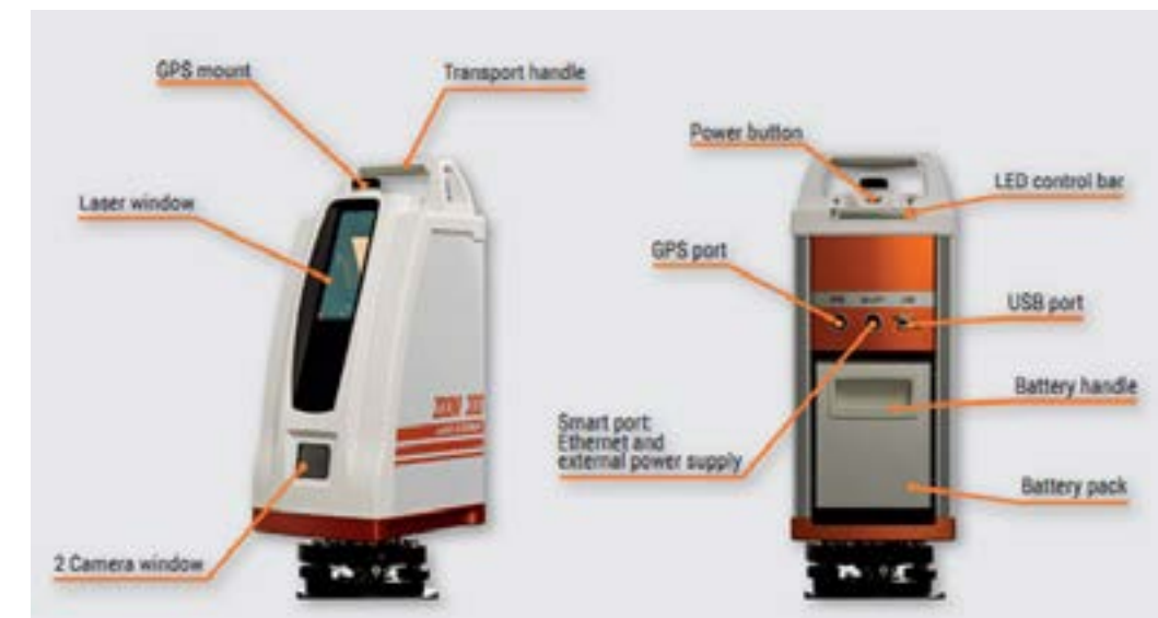
Figure 2. Laser Scanner Geomax SPS Zoom 300.
