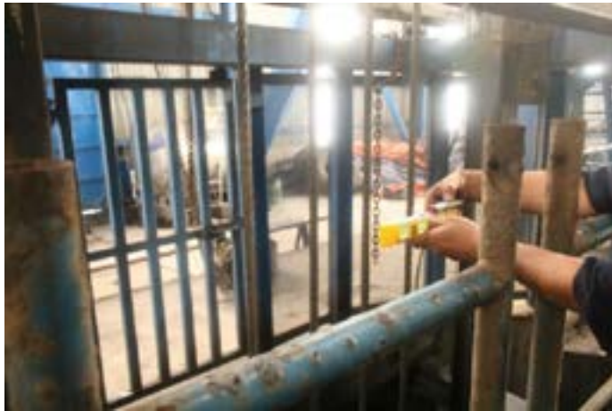
Figure 17. Measuring the distance between two shaft rail tracks or guides for accuracy assessment.
