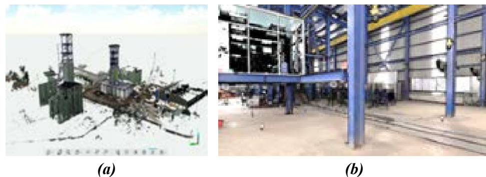
Figure 3. Result of TLS scanning for part 1: (a) Outside of the headframe; (b) inside of the headframe.
