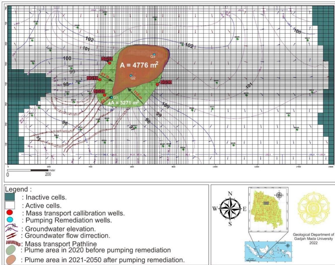
Figure 1. Recommended conventional pumping remediation in study area
