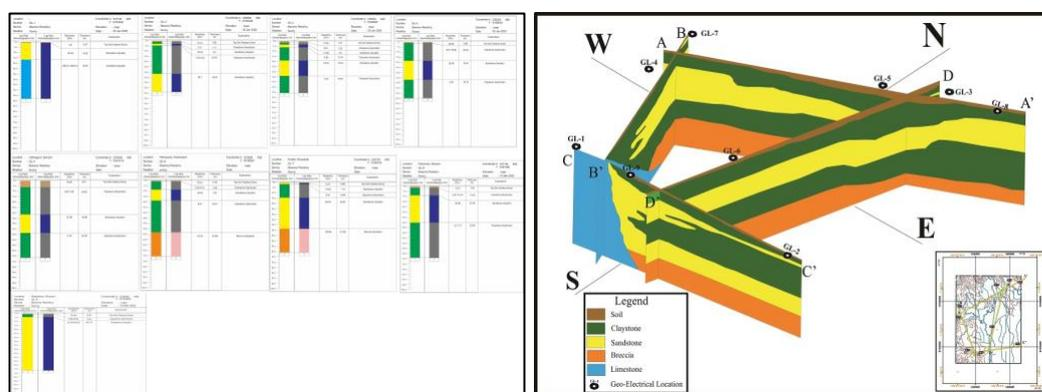
Figure 2. (a) Bore Hole Point 1-9; (b) Fence Diagram of Geoelectrical Field Measurement Result
