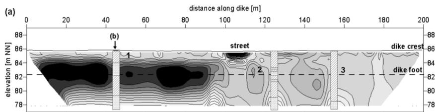
Figure 1. Resistivity image of a river embankment, showing sandy parts (weak spots by high resistivities (dark)).
