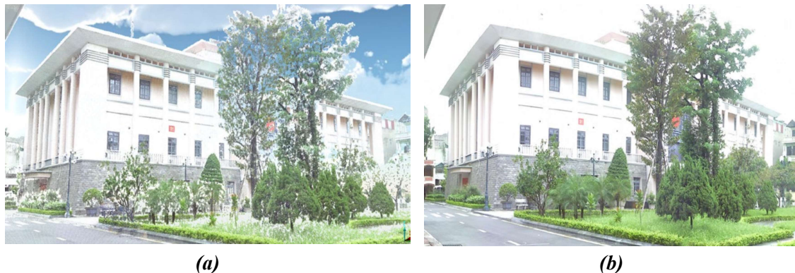
Figure 2: 3D model in the design and construction of civil works [70] ((a) Point cloud model; (b) Photo taken from a digital camera)
