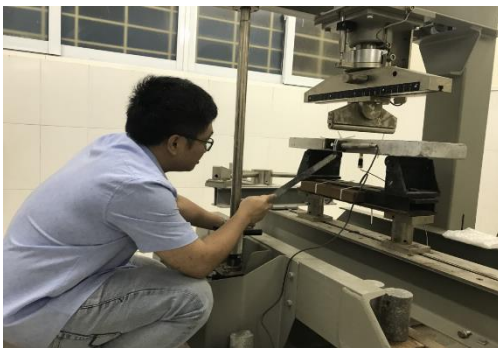
Figure 10. Testing of reinforced concrete sheeting. content.
