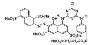
Figure 1: Structure of Synozol red HF-6BN
