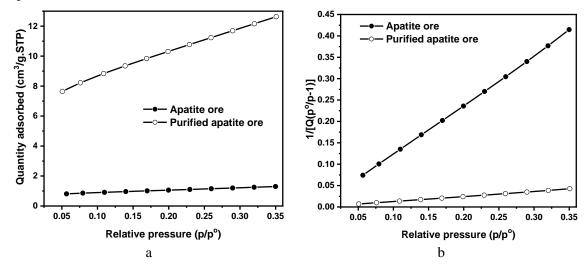
*Figure 4.* The  $N_2$  adsorption isotherm (a) and BET plot (b) of apatite ore and purified apatite ore.
