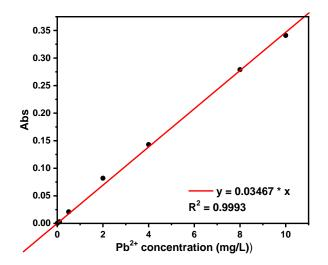
*Figure 16.* Calibration curve of Pb<sup>2+</sup> determined by AAS method.
