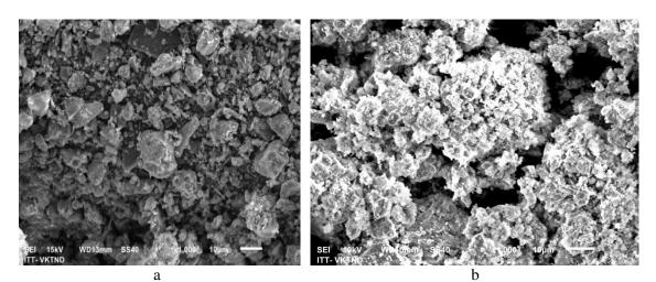
Figure 2. SEM images of apatite ore (a) and purified apatite ore (b).
