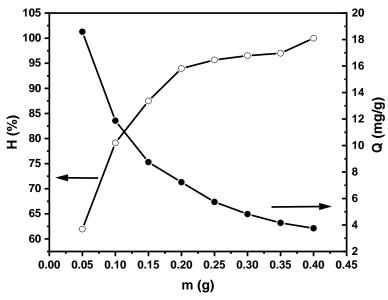
Figure 7. Variation of adsorption efficiency and capacity against mass of apatite ore (at  $pH_o$ ,  $C_o = 30$  mg/L, contact time = 45 minutes).
