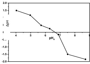
Figure 8. Graph for determining pH<sub>pzc</sub> of apatite ore.
