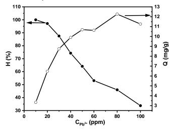
Figure 12. Variation of adsorption efficiency and capacity against  $Pb^{2+}$  ions initial concentration with  $m_{apatite} = 0.15$  g, pH<sub>o</sub>, contact time = 60 minutes.
