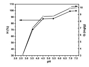
Figure 9. Variation of adsorption efficiency and capacity against pH with  $m_{apatite} = 0.15$ g,  $C_0 = 30$ mg/L, contact time = 45 minutes
