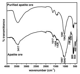
Figure 1. IR spectra of apatite ore and purified apatite ore.
