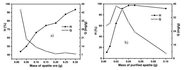
*Figure 17.* Variation of adsorption capacity (Q) and efficiency (H) against mass of apatite ore (a) and purified apatite ore (b) at  $C_0 = 30 \text{ mg/L}$ ,  $pH_0$ , t = 45 minutes with apatite ore and 15 minutes with purified apatite ore.
