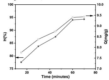
Figure 10. Variation of adsorption efficiency and capacity against contact time with  $C_0 = 30 \text{ mg/l}, \text{ pH}_0, \text{ m}_{apatite} = 0.15 \text{ g}.$
