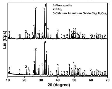
*Figure 14.* XRD patterns of apatite ore before and after Pb<sup>2+</sup> adsorption.
