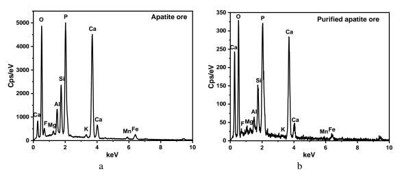
Figure 5. EDX spectrum of apatite ore (a) and purified apatite ore (b).
