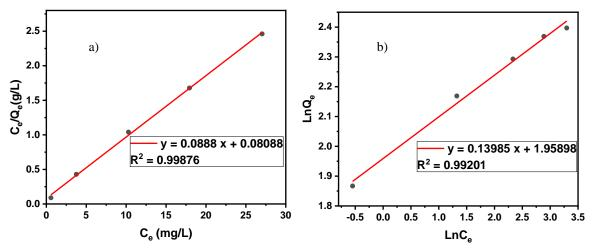
*Figure 13.* Adsorption isotherm curves of Pb<sup>2+</sup> against the Langmuir model (a) and Freundlich (b)
