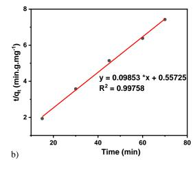
*Figure 11.* Adsorption data modeled using three kinetic models: (a) Lagergren's pseudo-first-order law, (b) McKay and Ho's pseudo-second-order law, and (c) the intra-particle diffusion model.
