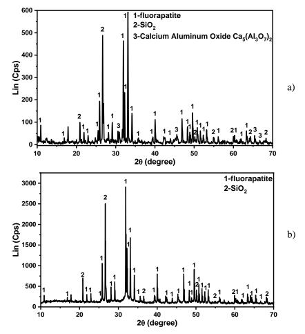
Figure 3. X-ray diffraction pattern of apatite ore (a) and purified apatite ore (b).
