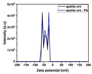
*Figure 15.* Zeta potential distribution of apatite ore before and after Pb<sup>2+</sup> adsorption.
