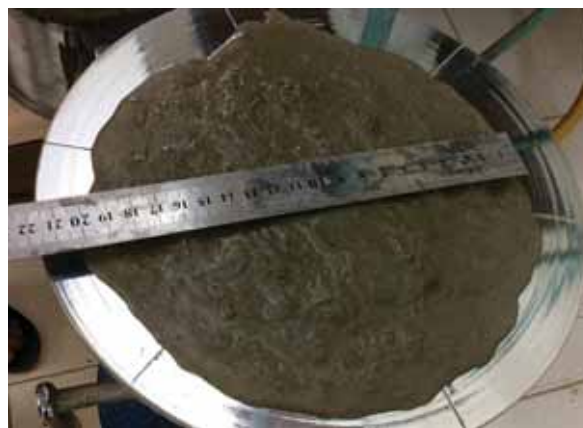
Fig. 5. Determination of workability of geopolymer concrete mixtures according to the cone flow diameter
