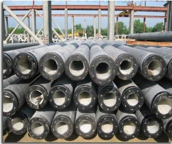
Figure 2. The PCCP piles with  $\Phi 300$ .
