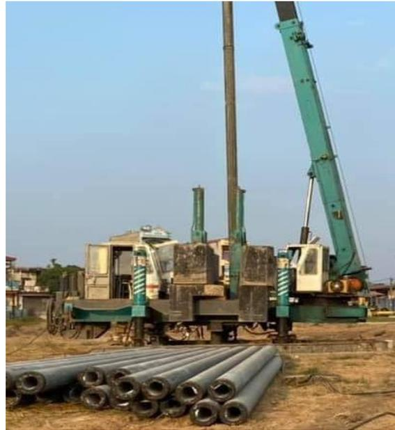
Figure 3. The pile driver ZYC180BS - B.
