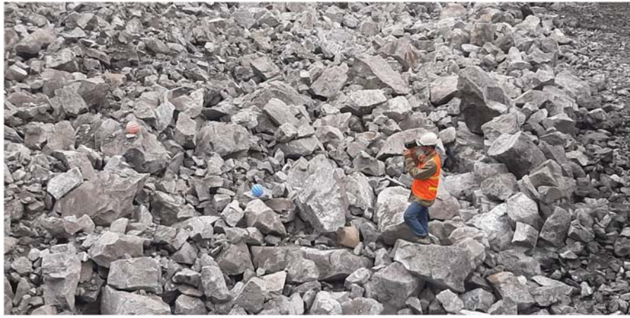
Figure 2. An example of image capture for blast fragmentation measurement. 'Images are available in colour online.'
