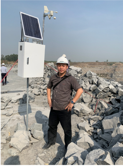
Fig. 9. Installation of the monitoring systems for temperature, humidity and wind speed at Nui Beo coal mine
