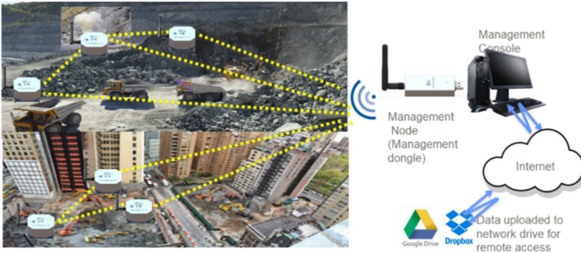
Fig. 3. Description of the wireless mesh networking for vibration monitor
