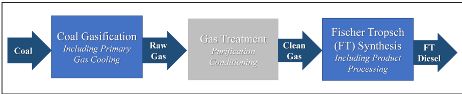
Fig. 1. Simplified Coal-to-FT diesel process chain
