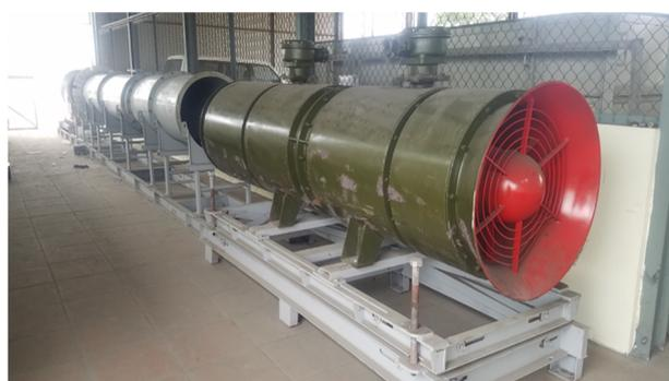
**Fig. 1.** Experimental apparatus for determination of duct resistance.
