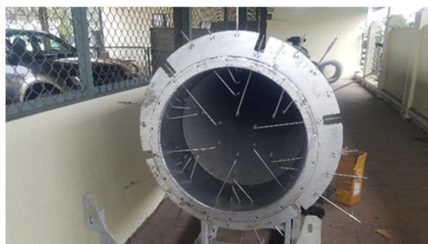
**Fig. 4.** Cross sectional area for pressure measurement and pitots.
