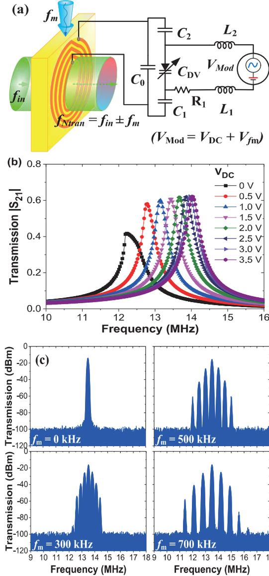
**Fig.2.** (a) The control circuit of the unit cell. (b) Resonance frequency responses of the unit cell as a function of the voltage control  $V_{DC}$ . (c) The transmitted power of the unit cell when are applied time-varying modulated frequency at 0, 300, 500, and 700 kHz.
