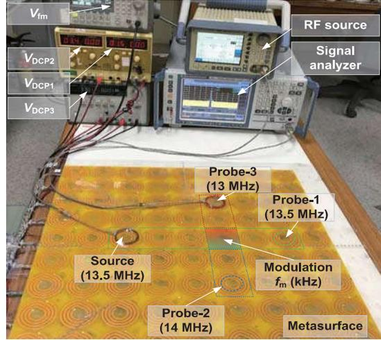
Fig. 5. The measurement system for multiple bandpass wireless power transfer.
