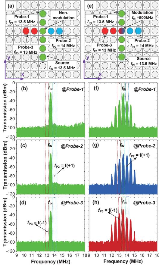
**Fig. 6.** The measurement of transmitted power. (a)-(d) the transmitted power from a wave source (13.5 MHz) to the probes without applying time-frequency modulation. (e)-(h) with using time-frequency modulation at 500 kHz.
