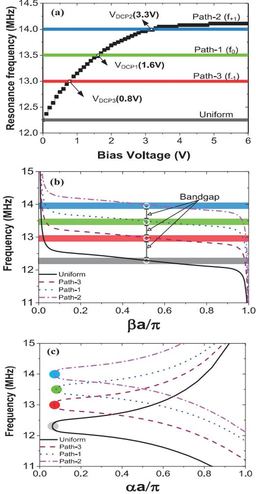
**Fig. 3.** (a) The illustration of three magnetic waveguides. (b) The response resonance frequency of the unit cells relates the DC voltage bias of the three paths and uniform region. (c) the propagation constant, and (d) attenuation constant.
