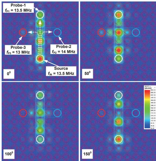
Fig. 4. The simulation results of the magnetic field distribution on the three paths at the phase of 0, 50, 100, and 150°.
