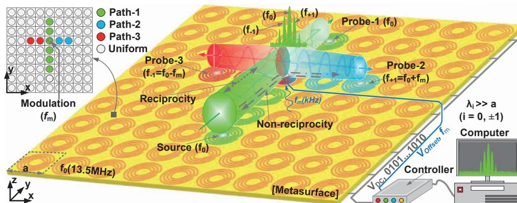
Fig.1. The schematic of time-frequency metasurface for multiple bands wireless power transfer system.
