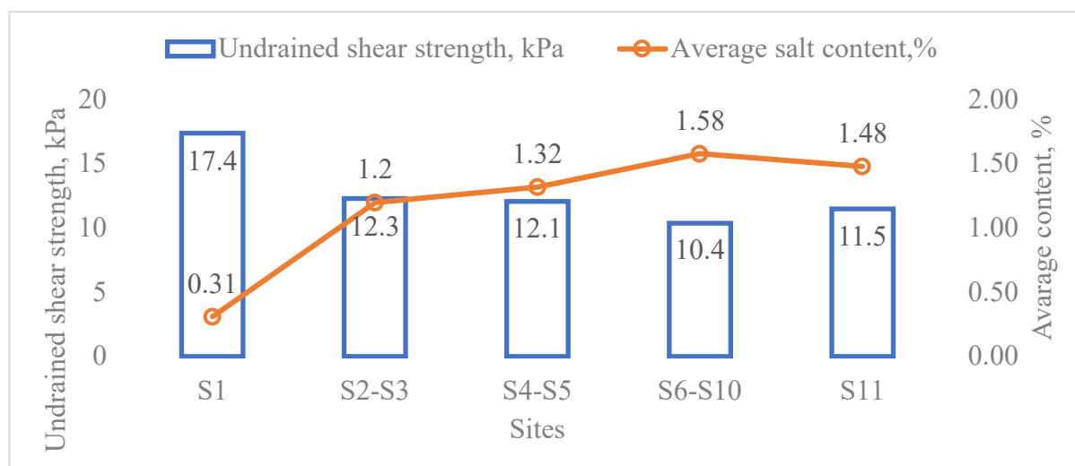
Fig. 4. The relationship between salt content and undrained shear strength obtained from UU test of soft soil
