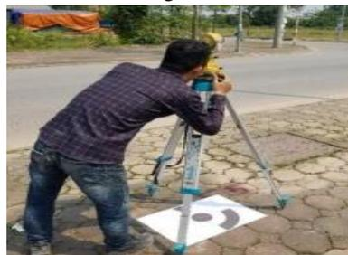
Figure 4b: Target on tripod legs
