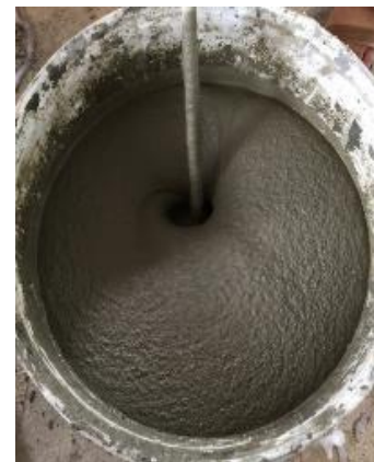
(c) Foam concrete mixture
