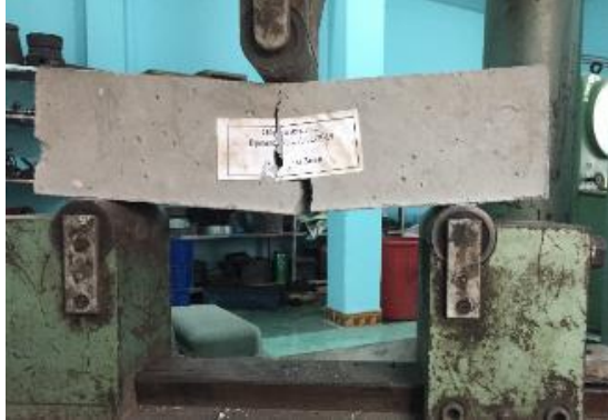
Figure 5. Testing flexural strength
