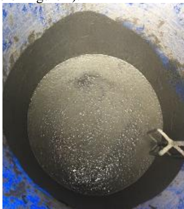
(a) Concrete mixture without foam
