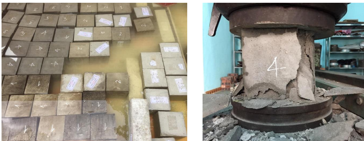
Figure 1. (a) - Foam concrete samples and (b) - Compression test sample
