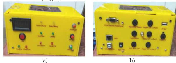
Fig.3. GNSS data receiver and transmission device a) Front ; b) Behind
